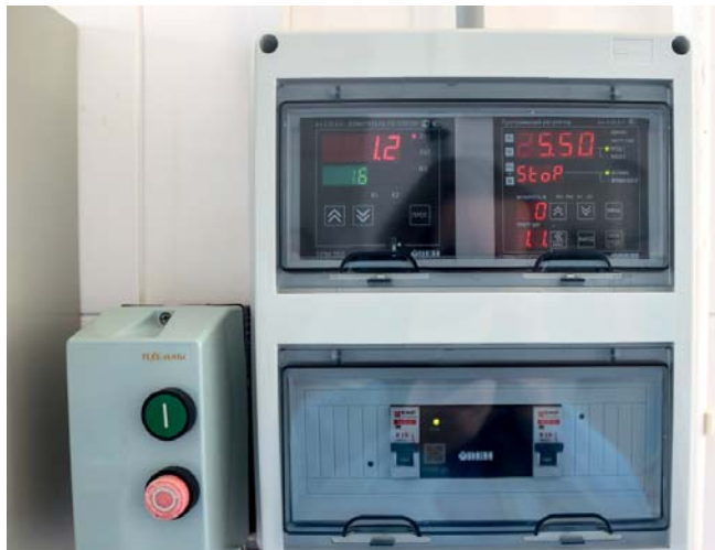
FIGURE 2. Device for online-monitoring of milk coagulation process
