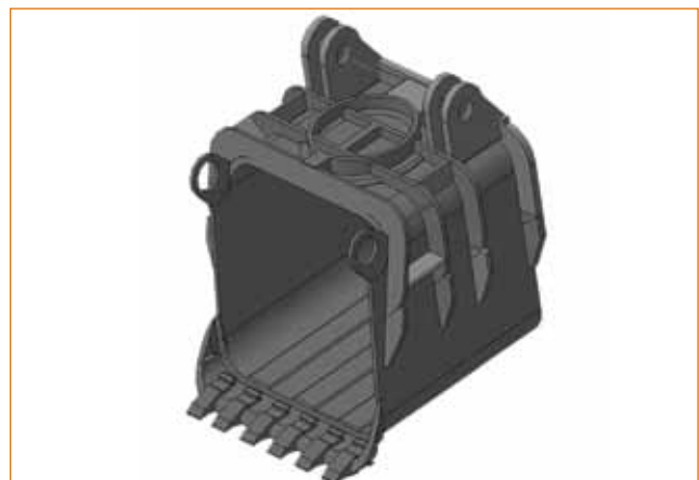
FIGURE 4 Model of the improved bucket of the EKG-10 excavator
